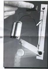
In this example one thin 100 μm (0.1 mm) diameter Muscle Wire®, powered by 3 volts at 200 milliamps, contracts by 4% of its length, and pulls with over 135 grams to lift the lever and weight. Remove power and the wire relaxes, ready for millions of cycles more!
